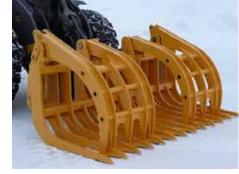
with ease, as well as unload and sort product quickly. Grapples of all shapes and sizes are available as well as custom-built models.
